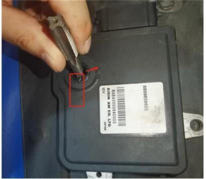
After manually adjusted TCM spare part groove direction, it could be installed on the vehicle at N gear status.
