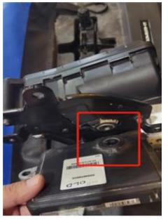
In view of this, reinstalled the old TCM (with the groove facing P), started the vehicle, engaged the EPB, shifted to N gear, after that, long pressed the SSB switch to turn off the engine (note: in N gear, short pressing the SSB switch cannot turn off the engine), and then remove the TACM and the old TCM.
