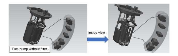
Type 2: Fule filter is integrated with fuel pump
