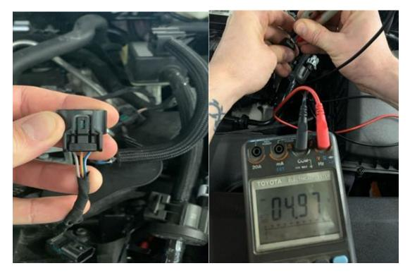
5. Checked the engine control unit plug. found a weak contact in the engine control unit pad. After replacing the pin, the problem was solved.
