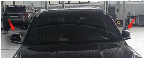
5. Since the part is good, we thought that the cause maybe the software and confirmed with R&D. The reason is that, if the running current is greater than 70% of the starting current and the duration is greater than 300ms, the module will determine the stop position and then power off. The fault mainly occurs in winter. Due to the increase in motor operating current at low temperatures, the
