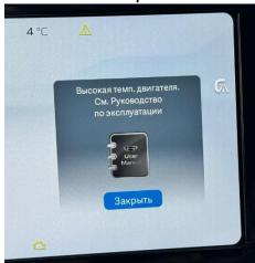
2. Used GLDS to check DTC, found ECM-P021700 Engine Coolant Overtemperature Condition.
