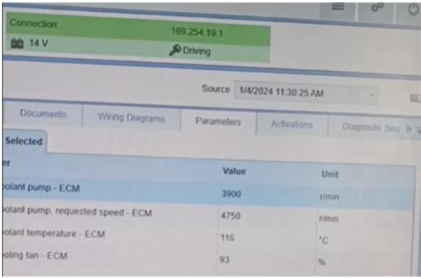
4. Maybe some problem with the pump, then checked the fan of water pump, it was stuck.
