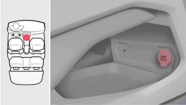
Power outlet in the front tunnel console
