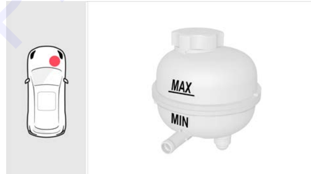
high voltage battery coolant expansion tank
