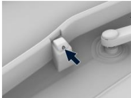
Illustration: cleaning the wiper spray head
