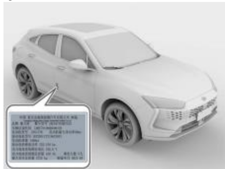
Figure: nameplate position of the whole vehicle (the picture position is for reference only, and the specific situation shall be subject to the actual vehicle)
