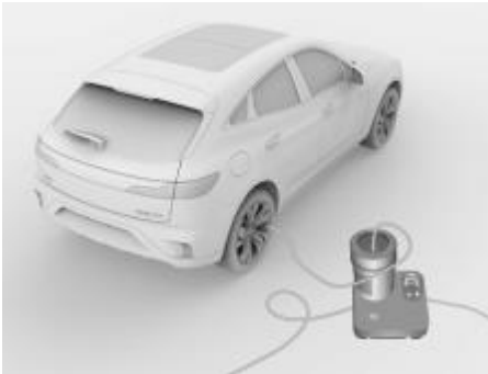
Figure: install tire repair rubber tank
