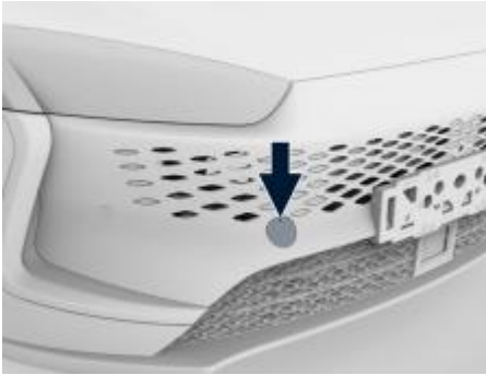
Figure: remove the front towbar hole plug
