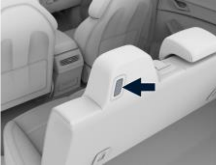
Picture: The unlocking device is located on the rear side of the outer rear headrest
