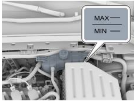
Figure: water storage bottle assembly (front compartment trim cover removed)
