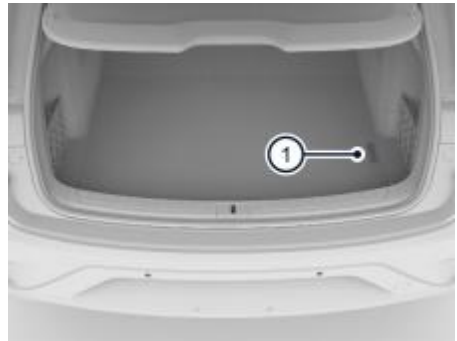
Figure: vehicle VIN code position (picture position is for reference only, please refer to the actual vehicle for specific conditions)
