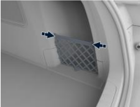
Figure: remove the rear side wall net pocket 1. Press both sides inward, disengage the mesh bag clip, and remove the rear side wall mesh bag.
