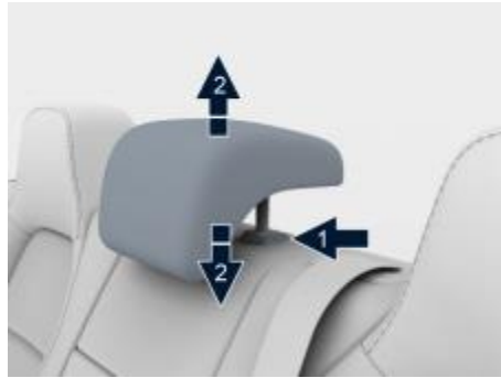
Picture: Adjusting/removing the head rest
