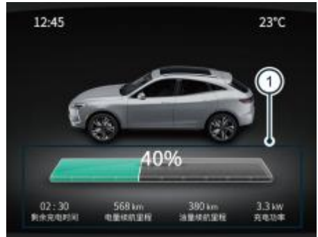
Illustration: The meter displays charging information. When the charging is completed, the charging interface indicator light stops flashing and turns steady green, and the meter or touch screen displays the charging completion message.
