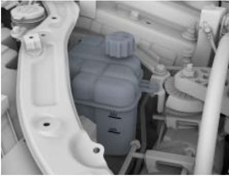
Figure: auxiliary water storage bottle assembly (front compartment trim cover removed)
