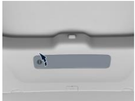
Figure: triangle warning sign is on the trim panel of back door
