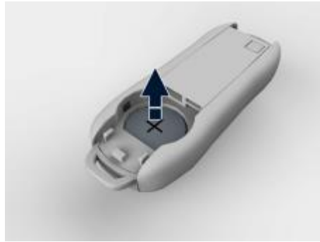
Illustration: remove the remote key battery
