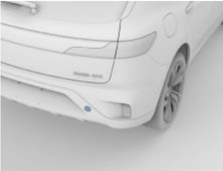
Figure: Removing the rear trailer hitch hole plug cover
