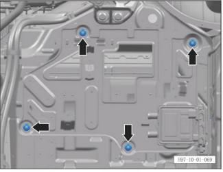
b. Unscrew 4 fixing nuts of the water heating PTC assembly bracket.
