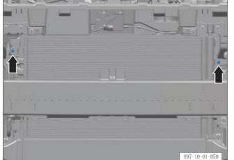
b. Unscrew 2 fixing bolts of the condenser.
