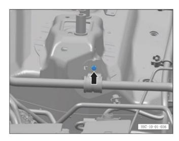
b. Unscrew the fixing bolts of the front evaporator outlet pipe assembly.
