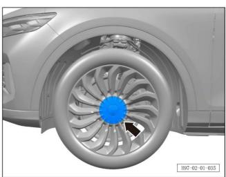
• Type II of the rim trim cover: take out the rim trim cover, and install it on the rim. After the installation is completed, confirm that the clamping is secured and check the flush between the rim trim cover and rim.
