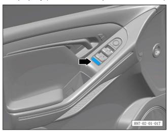
Check the function of the POT switch (turn off the POT switch after the inspection is passed).
