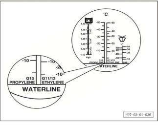
b. Read the freezing point value of coolant
