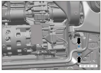
n. Check the 2 fixing nuts of the rear stabilizer bar. Tightening torque of nut: 30±5Nm.
