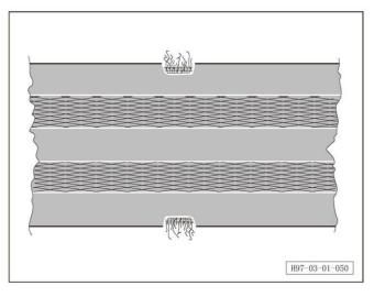
d. The seat belt must be replaced when the fabric loop on the edge is torn.
