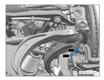
m. Check the 2 fixing bolts of the front caliper bracket. Tightening torque of bolt: 120Nm + 45°.
