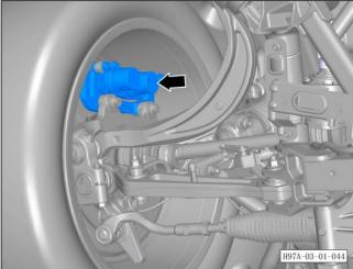
i. Replace the brake fluid for the left front brake wheel cylinder until the brake fluid is renewed.
