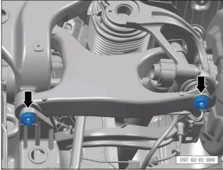
h. Check the 2 fixing nuts of the lower swing arm assembly.
