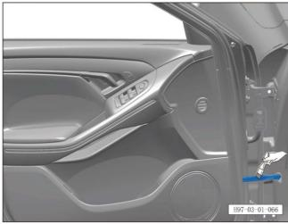
c. Use a small brush to apply the specified grease to the upper and lower sides of the sliding surface of the stopper.
