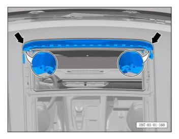
b. Clean the debris at the sunroof front drain hole and sunroof rail, and check whether the drain hole is blocked.
