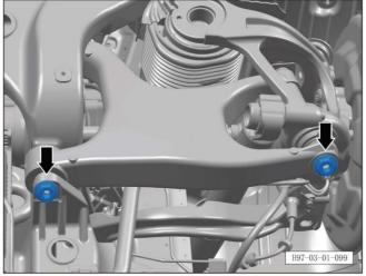
h. Check the 2 fixing nuts of the lower swing arm assembly.
