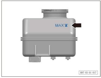
I. Add brake fluid to the level indicated by the arrow on the "MAX" mark of the reservoir.
