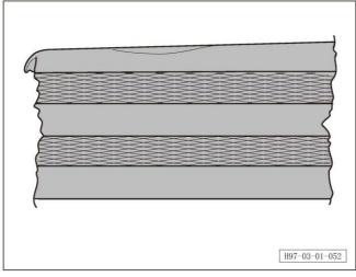
f. The seat belt must be replaced when one side of the seat belt is deformed or the edge of the seat belt is wavy.
