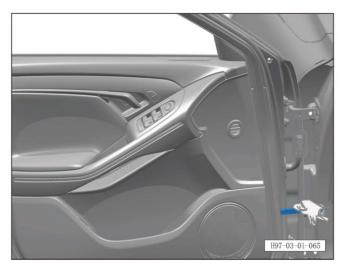
b. Use a soft cotton cloth to remove dirt from the surface of the black pull rod of the stopper.
