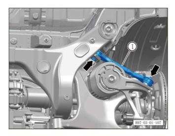
p. Tighten the 2 fixing nuts of the rear toe-in arm assembly  $\ensuremath{\mathfrak{D}}.$
