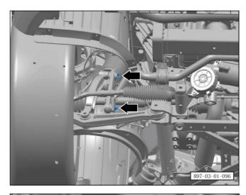
d. Check the 2 fixing nuts of the front stabilizer bar tie rod.
