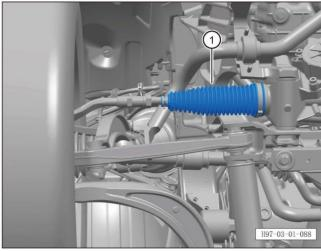
d. Check whether the steering gear rubber dust cover ① is damaged. If so, replace the steering gear rubber dust cover. See 6.1.6.6 Removal and refitting of steering gear dust cover
