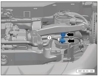
o. Check the 2 fixing nuts of the rear stabilizer bar tie rod assembly  $\mathbin{\textcircled{\scriptsize 1}}$ .
