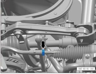
k. Check 1 lock nut connecting the steering gear outer ball joint to the steering gear assembly.
