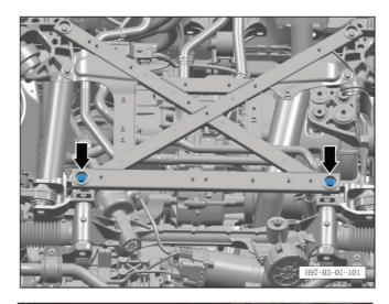
j. Check the 2 fixing bolts of the front subframe.Tightening torque of bolt: 115Nm+90°.
