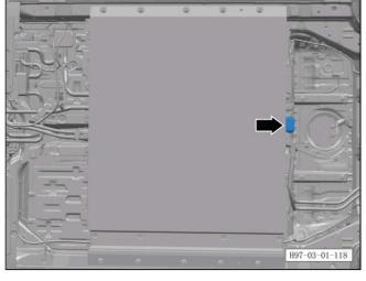
b. Lift the vehicle and turn off the manual service switch.
