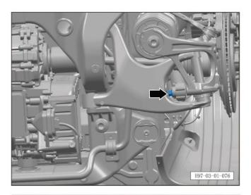
s. Tighten the 2 fixing bolts of the rear shock absorber assembly and the rear steering knuckle.
