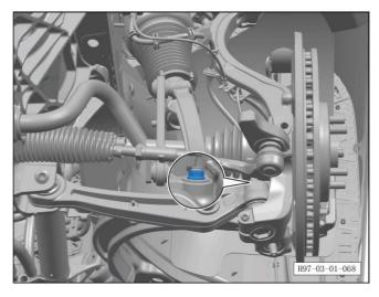
f. Check 1 fixing nut connecting the lower control arm ball joint to the steering knuckle.
