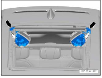
b. Clean the debris at the sunroof rear drain hole and sunroof rail, and check whether the drain hole is blocked.
