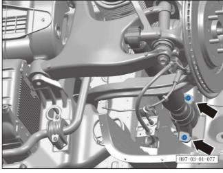
t. Tighten the 2 fixing bolts connecting the rear strut assembly  $\ \ \, \bigcirc \ \,$  and the body.
