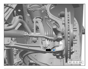
g. Check 1 fixing bolt connecting the lower control arm to the steering knuckle.
