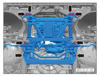
I. Check the 8 fixing bolts connecting the front subframe to the body.
