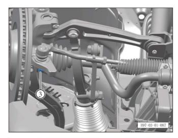
c. Check whether the tie rod ball joint fixing nut ③ is secure.
