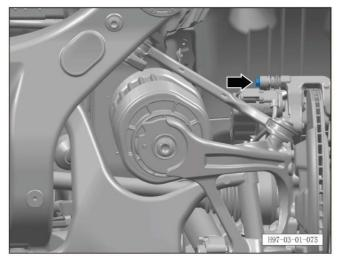
r. Tighten 1 fixing bolt of the rear caliper bracket.
