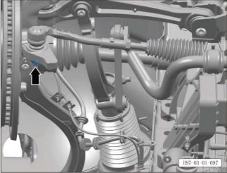
e. Check 1 fixing nut connecting the steering gear outer ball joint to the front steering knuckle.
