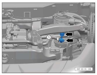
o. Check the 2 fixing nuts of the rear stabilizer bar tie rod assembly  $\mathbin{\textcircled{1}}$ .
