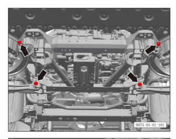
j. Check the 4 fixing bolts of the front subframe. Tightening torque of bolt: 115Nm + 90°.
