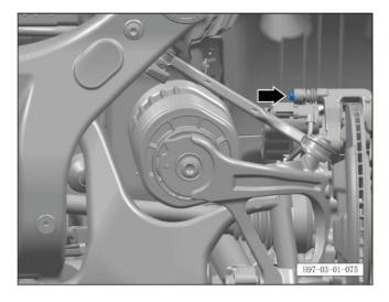
r. Tighten 1 fixing bolt of the rear caliper bracket. Tightening torque of bolt: 120Nm + 45°. 3. Maintenance Manual 3-99 Maintenance
