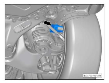
k. Replace the brake fluid for the left rear brake wheel cylinder until the brake fluid is renewed.
