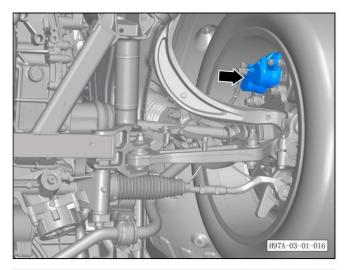
h. Replace the brake fluid for the right front brake wheel cylinder until the brake fluid is renewed.
