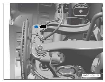
i. Check 1 fixing bolt of upper swing arm and steering knuckle.
