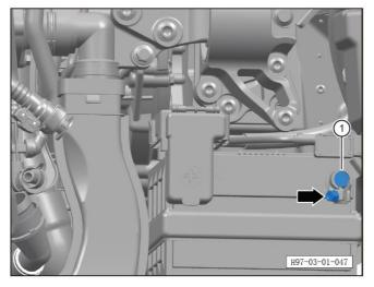
4. If the vehicle is parked for a long time, disconnect the battery negative terminal.
