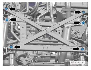
I. Check the 6 fixing bolts connecting the front subframe to the body.
