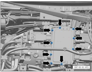
b. Check whether the 9 fixing bolts of the engine compartment high-voltage box are firm.
