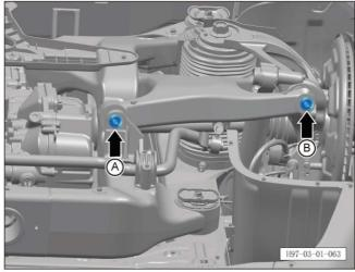
q. Tighten the fixing nut A and bolt B of the rear lower arm assembly.
