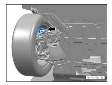
k. Replace the brake fluid for the left rear brake wheel cylinder until the brake fluid is renewed.
