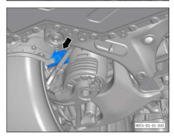
j. Replace the brake fluid for the right rear brake wheel cylinder until the brake fluid is renewed.
