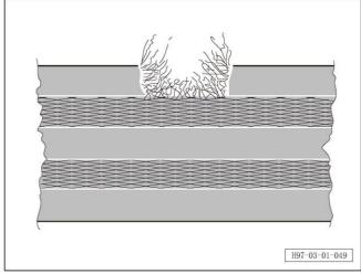
c. The seat belt must be replaced when it is broken, torn or scratched.
