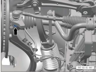
e. Check 1 fixing nut connecting the steering gear outer ball joint to the front steering knuckle.
