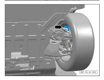
j. Replace the brake fluid for the right rear brake wheel cylinder until the brake fluid is renewed.
