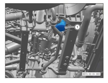
c. Tighten the engine oil filter ① using the oil filter removal & refitting tool.
