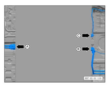
c. Disconnect the front high voltage harness A, rear high voltage harness B, and connector C of the body harness.
