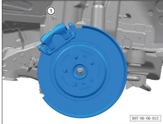
f. Remove the rear brake assembly and brake caliper assembly  $\mathbin{\textcircled{\scriptsize 1}}.$
