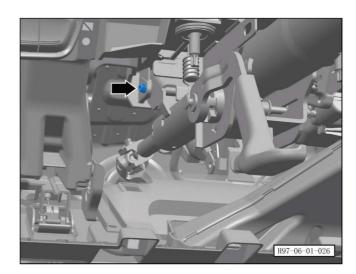
b. Unscrew 1 fixing bolt of the upper steering shaft. Tightening torque of bolt: 20±3Nm.
