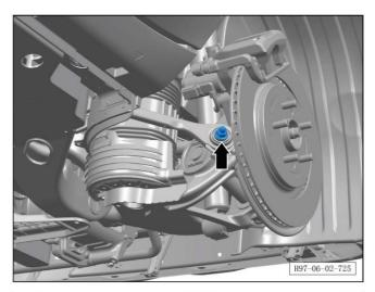
b. Remove 1 fixing nut of the rear toe-in control arm assembly and pull out the bolt.
