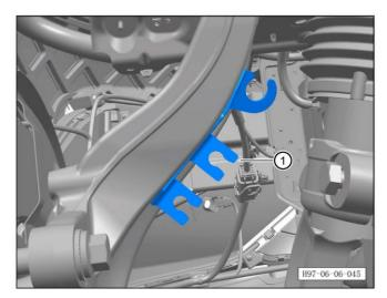
c. Take down the front wheel speed sensor bracket  $\widehat{\mbox{\Large $1$}}.$
