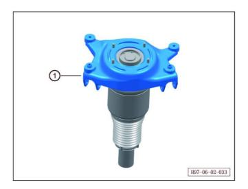
b. Remove the reinforcement seat  $\ensuremath{\ensuremath{\mathbb{Q}}}$  on the front shock absorber.
