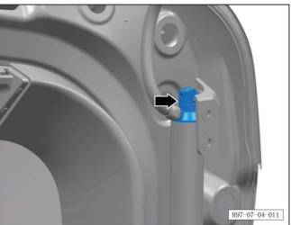
b. Pry up the spring clip (at the body) with a screwdriver and disengage the left POT strut.
