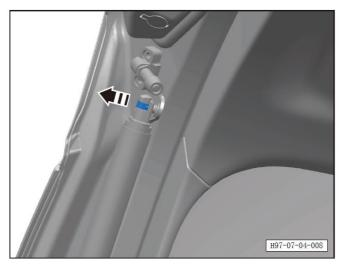
c. Pry up the spring clip (at the tailgate) with a screwdriver as indicated by the arrow.
