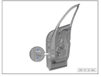
b. Unscrew 2 fixing screw of the front door stopper (at the door).
