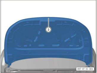
f. Remove the engine hood assembly ③.
