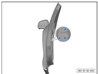
d. Unscrew 3 fixing screws of the left front door lock body.
