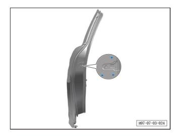
c. Unscrew 3 fixing screws of the left rear door lock body.
