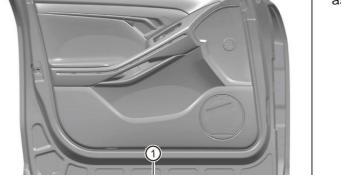
b. Disengage the left front door antifouling strip assembly ①.
