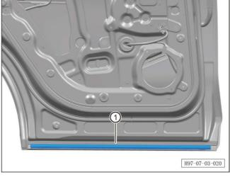
b. Remove the left rear door antifouling strip assembly  $\widehat{\ \ }$   $\widehat{\ \ }$  .
